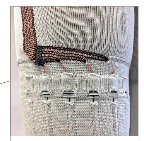
Fig. 4: Bandage with conductor tracks and integrated sensor threads
